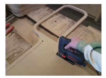
Now, just like I did when I was cutting out the outsides using the jig saw I have done the same for the insides, making sure that I was only 3mm away from the proper line. Once this was done the inside is ready to be routered.
