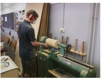
The final touch of giving the wood a quick sand left the corner of the jig a clean finish. Because of the dust that is created when using the lathe I make sure that I am wearing the correct safety equipment, dust mask so I don't inhale too much dust, glasses to protect my eyes, earmuff for my ears and of course covered shoes for my feet.
