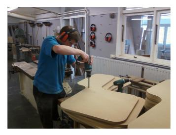
This time before I use the jig saw to cut beside the line roughly, I needed to drill a hole in each end for blade so that it can actually cut the outside. This took a while as I had to cut 48 different holes.
