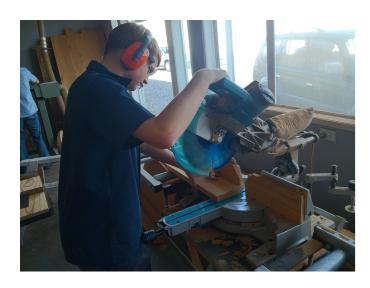
Here I am using the drop saw to cut out the sides of the jigs, making them the correct size. I am wearing earmuffs and glasses to protect my eyes and ears from the loud noise and possible fragments of wood.
