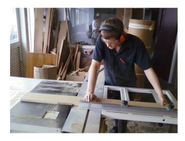
In this picture I am cutting the kerfs in the wood, allowing it to be pliable and able to be bent around the jig. To do this correctly I had to carefully mark out where the kerfs would be cut and make sure that the wood was square with the fence when I was cutting them. Also I had to make sure that I was being safe with the saw and that I had my hands a safe distance away and earmuffs and glasses on.
