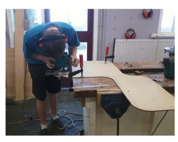
Next I had to cut out the inside. I did this by routering the inside edges using a small router which had a fence on it. This kept it the same all the way around. This meant that all of the straight edges had been completed. Again all the safety equipment that was needed was worn including shoes, earmuffs, glasses and a face mask.
