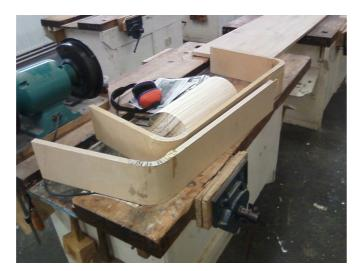
In the end the method didn't work well at all, some of the kerfs split and the corners didn't go tightly around the corners. I couldn't work out why, as it had gone well in the previous tests. Then I realised that I had made a stupid mistake and confused radius and diameter and ending up making it half the size needed. This meant that I had to start again...
