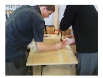
Them I put the jig and the method on a full side scale test. I put gladwrap down to protect my jig from the glue setting on it, then clamped the custom wood to the jig, along with a rope mechanism to keep it tight around the corners. Then the kerfs were filled with glue.
