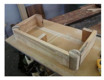
Then the other pieces of the jig were cut out. The wide bits of pine were cut with a 45 degree angle so that they would fit snugly to the corner pieces. These were cut carefully on the table saw, using safety glasses, earmuffs and shoes to protect my eyes, ears and feet. Once the side had been screwed in they were reinforced with another piece of wood to keep it square when in got glued together.
