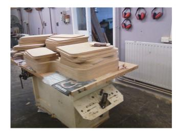
Now that all of the pieces are cut out to the same size they are ready to be glued together. The method that I used was to put a layer of glue between the 6 pieces then add weight (the off cuts) to hold it together as the glue id left to cure. It was easier to glue the pieces together in smaller parts to make sure they were in line with another.
