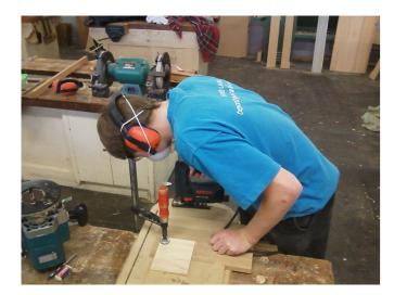
Here I am using the jig saw to cut the corners of the jig roughly, before spoke shaves and sandpaper is used to finish it off. Once the jig is perfect the inside edge is coated with resin to make it harder and more hard wearing.
