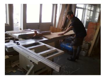
Now I got ready to cut out the sides of the mirror. I found some old custom wood that would be suitable and used the table saw to cut it down to 130mm width. Making sure that the edge was flat against the fence and my fingers were a safe distance away from the saw.
