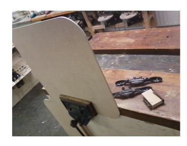
Next I had to shape the curves using sandpaper and the two different spoke shaves. Then the final thing that needed to be done to the jig was to coat the edges with resin so that they would become harder and more hardwearing.
