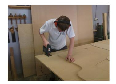
The next job that I had to complete was cutting out 24 pieces to be routered so that it would end up with the correct thickness once they were glued together. I marked out 4 outlines on each sheet of custom wood and then used the jig saw to cut an outline 3mm around the line.
