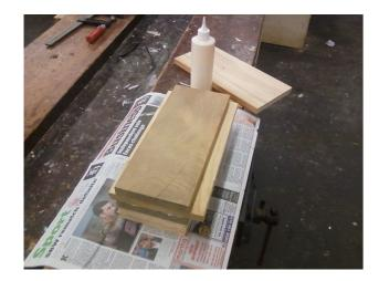
The first part of the construction is building the jig that will be used to bend the wood around. The curved part will be made on the lathe. For this part a few off cuts of pine will be used and glued together to get the required thickness.
