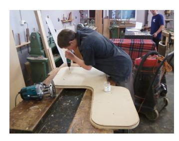
Now it was time to start routering the gaskets to the exact shape that is required. The jig was screwed into the 18mm custom wood, then clamped in place. The router had the copy cutter tool on the edge of it so it copied the jig every time. This meant that by the end I had 24 copies of the jig. A vacuum cleaner was used when I was doing the routering so that the dust wouldn't go everywhere.
