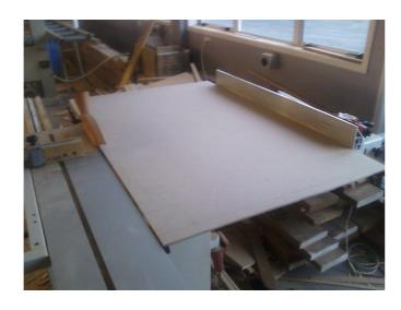
The first thing that I had to do was mark out the design on a piece of 6mm custom wood. This would become the jig that is used to cut out the 'gaskets' that would be glued together to make my final product. The custom wood was cut to size using the table saw.
