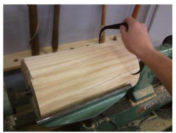
I started again by gluing some pieces of pine together and turning in on the lathe, this time to the correct thickness of 164mm. This would mean that the outside radius of the wood would be 100mm. Which is the same as what I had designed.
