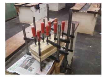
These were all cut to the same length before they were glued together. With a layer of PVA aliphatic glue inbetween each piece they were clamped in place using 8 F clamps and left to dry so the glue will cure.
