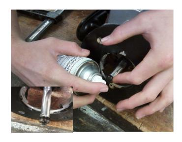
One of the problems that occurred when I was using the router was that after I had done a few pieces the bearing started to seize up, this meant that it cut into the jig a little. (Which would be something that I would have to sand out later). After I had realised the problem I made sure that the bearing was well lubricated so that it wouldn't happen again.
