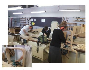
Now that all of the pieces had been glued together it was time to let the sanding process begin. The main focus was to get the inside flat so all 4 pieces could be glued together. To speed up this process I got some of my friend to help out so that this job could be finished before term 4. Where the pieces were out of line builders fill was used to fill in the gaps.
